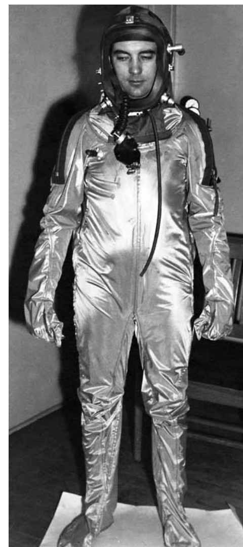
John Flagg shows the bladder of the Model 3 in March 1950. The designers uncoupled the outer restraint layer from the gas container in an attempt to increase mobility. The unusual clear-plexiglass helmet of the earlier suits gave way to a modified partial-pressure suit helmet with a face seal.
