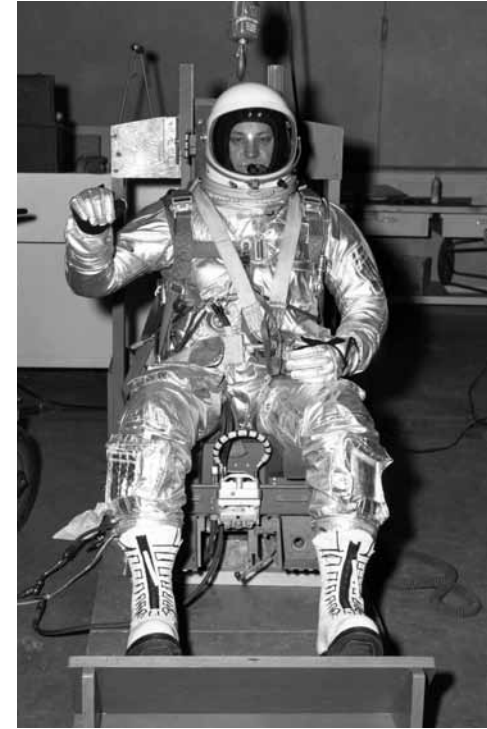
A David Clark Company S901J suit with the original silver exterior cover. S901J suits were later retrofitted with white, then brown exterior covers in an attempt to reduce cockpit instrument washout from sunlight reflecting off the suit.
