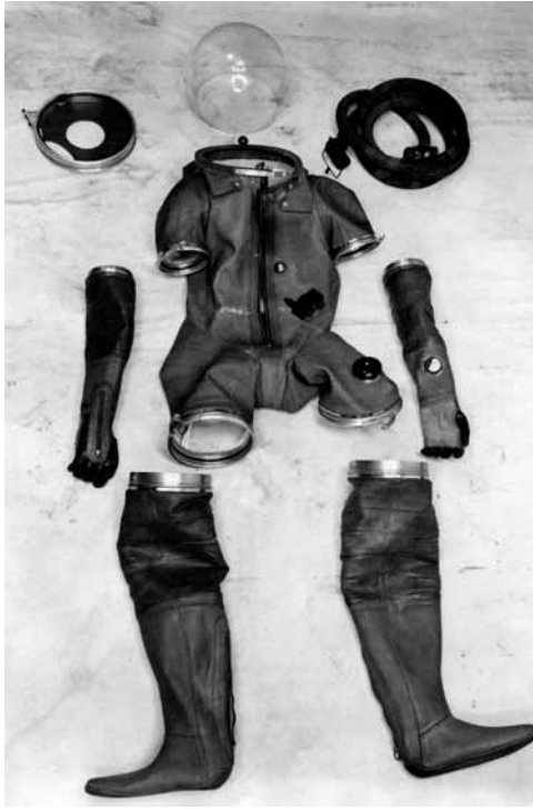
The B.F. Goodrich Type 5E Strato-Suit weighed 22.5 pounds and was significant in having detachable arms and legs, allowing a certain amount of tailoring for the individual. The neck seal for the helmet is shown at top left.
