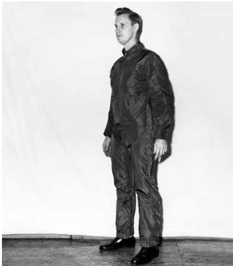
This is the David Clark Company version of the Z-2 G-suit. Note the zippered pockets on the shins, chest, and sleeve. Sometimes it seemed as if the location and shape of the pockets were as important as the acceleration protection provided by the bladders hidden inside the suit.
