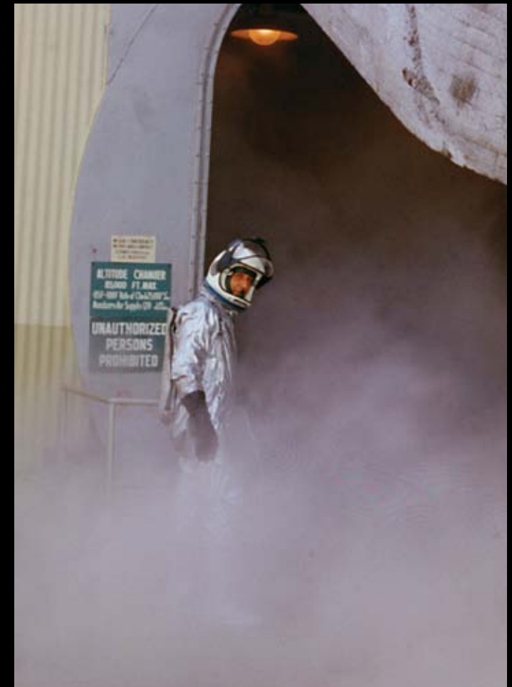
Another legendary test pilot, A. Scott Crossfield shows off an early David Clark Company MC-2 full-pressure suit in front of the Wright Field altitude chamber. The sign indicates the chamber was limited to 85,000 feet. Of note is the thickness of the raised entry door. – National Archives College Park Collection
