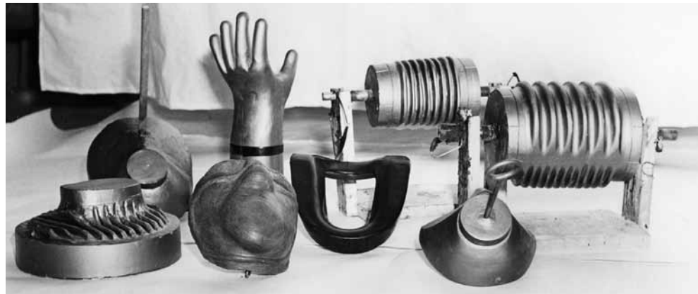
Above: The Model 8 was mostly a minor evolution of the Model 7, but included a large dome helmet that greatly improved comfort and allowed a much better range of head motion. Unfortunately, the plexiglass dome was too large to fit into most fighter cockpits and was soon abandoned.
