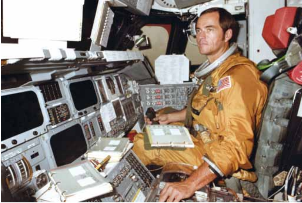
NASA astronaut Robert L. “Crip” Crippen in the cockpit of Columbia (OV-102) on October 10, 1980, prior to the launch of STS-1. Note the modified Lockheed SR-71 ejection seat and Crip’s David Clark Company S1030A full-pressure Ejection Escape Suit. Columbia was the only space-rated Orbiter to use ejection seats, and they were only active for the four orbital flight test (OFT) missions (although they were physically installed until after STS-9).
