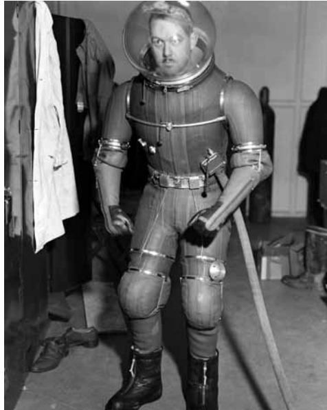
B. F. Goodrich developed the XH-1 suit, part of a series of increasingly better suits that were ultimately judged the best of the World War II efforts. Bellows at the elbows and knees provided improved mobility. Note the metal rod stretching between the shoulder rings, an attempt to control side-wise ballooning. This would become a feature on most of the subsequent suits designed by Russell Colley.
