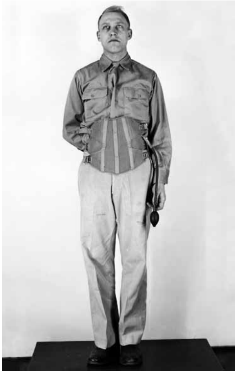
In 1932, LT John R. "Jack" Poppen, a naval flight surgeon, developed what became known as the Poppen Belt to fight the effects of acceleration. The concept was valid, but the belt needed to be inflated using a hand bulb (shown) in advance of being needed (a technique not well suited to the flight environment). A later version of the device was featured in the 1941 movie Dive Bomber .
